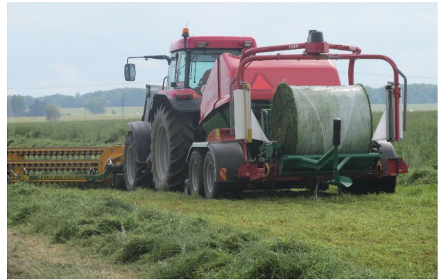
Forage is swathed, pressed to round bales and the bales are wrapped by an aggregate. Photo by Raivo Vettik
