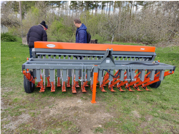
Direct drill "Underhaug" used for hay seeding in grassland renewal. Photo by Sirje Tamm
