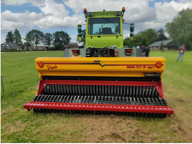
Seed drill "Vredo" for over-seeding used in grassland renewal. Photo by Sirje Tamm
