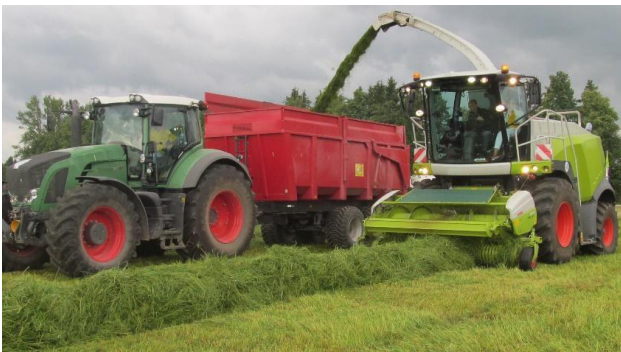
The collection and chopping of forage for silage by a self-propelled grass harvester. Photo by Raivo Vettik.
